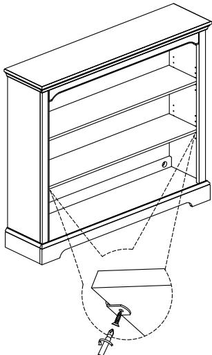
To adjust the shelf, release the screw from the bottom as shown.
