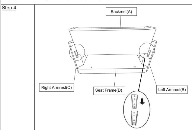
Slide the Tapered Connectors on the Backrest(A) into the Tapered Connectors on the Left Armrest(B) and the Right Armrest(C) as shown above.
