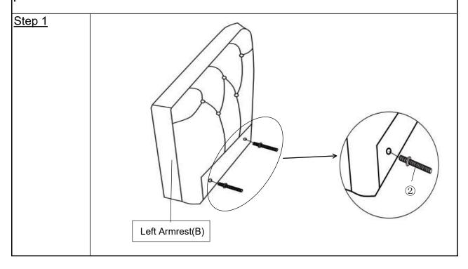
Screw the Screw Arbor(②) into mounting position on the Left Armrest(B) by hand until tight. Repeat the same step with the Right Armrest(C). Step 2 Right Armrest(C) Left Armrest(B) Seat Frame(D) Install the Left Armrest(B) and Right Armrest(C) to the Seat Frame(D) as shown above. Step 3 Left Armrest(B) Right Armrest(C) Seat Frame(D)
