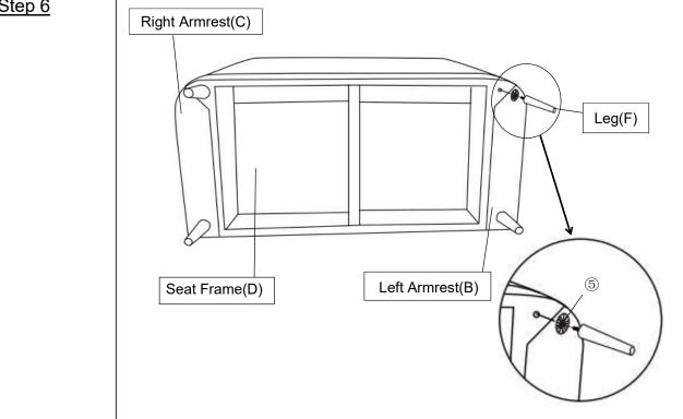
Install the Leg(F) into the bottom of Left Armrest (B) and Right Armrest(C) by placing Plastic Washer(⑤) on the threaded stem. Then insert threaded stem into the threaded mounting postion at the bottom of Left Armrest(B) and Right Armrest(C).
