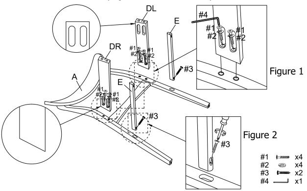
Step 2 . Attach front leg (part C) to side rails (parts DL & DR) and stretchers (part E) using bolts (part #1), spring washers (part #2), screws (part #3), allen wrench (part #4) and phillips head screwdriver.
