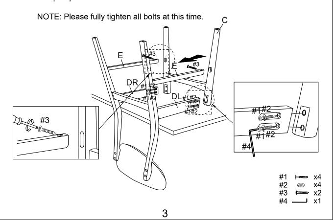
Step 3 . Attach seat (part B) to side rails (parts DL & DR) using screws (part #3) and phillips head screwdriver.
