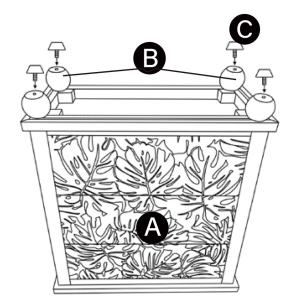
Flip the table assembly upside down. Attach the legs to the table assembly. Attach the leveling feet to the legs.
