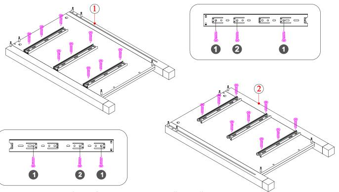
• Refer to the illustration to fix the Slide rails to theboard #1 and #2 with screws.
