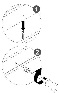
• Refer to the illustration, already assembled #4,#5,#6 on the panel #1 and #2. Then tighten the cam lock.
