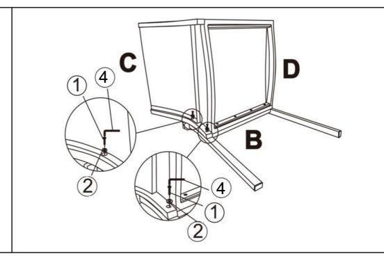
Attach Backrest(C) to Right Armrest/Leg(B) using Bolts(1) and Washer (2) with Allen Key(4)as shown above.
