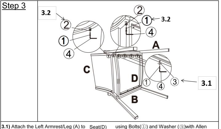
Key(4) as shown above. **3.2)** Attach the Left Armrest/Leg(A) to Backrest(C) usingBolts(1) and Washer(2) with Allen Key(4).
