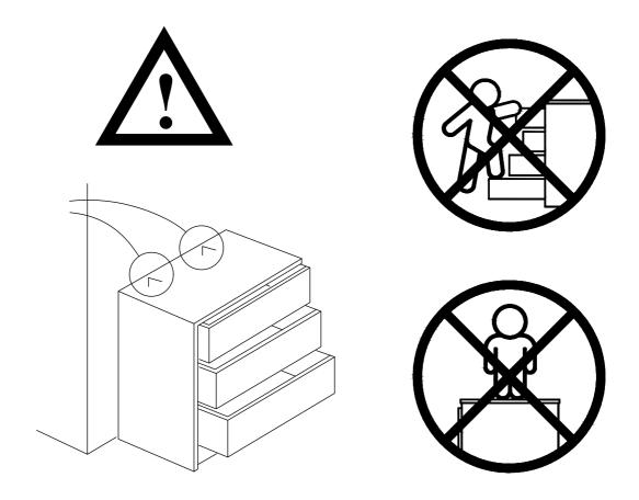
IMPORTANT: THIS UNIT MUST BE SECURE TO THE WALL TO HELP PREVENT TIPOVER. FOLLOW THESE INSTRUCTIONS TO INSTALL THE ANTI-TIPPING SAFETY BRACKET PROVIDED WITH THIS PRODUCT.
