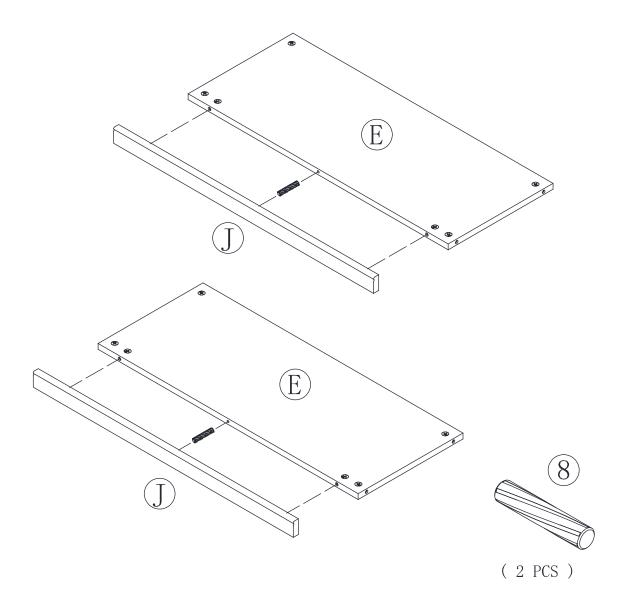
♦ Fasten the SHELVES (E) to the UPPER LEFT END (C). Tighten four HIDDEN CAMS
