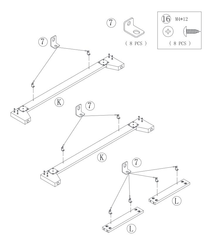
♦ Faten two SHORT BRACES (L) to the FEET (Y and O). Tighten eight HIDDEN CAMS
