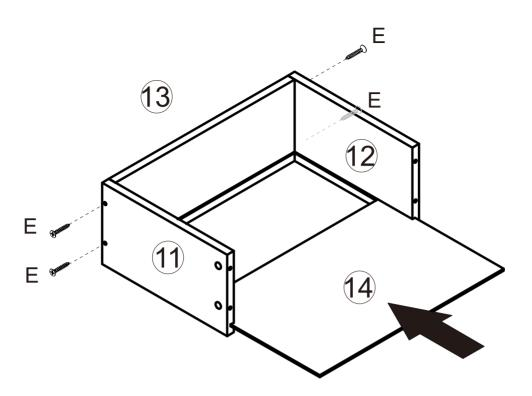
Connect board 13 to 11&12 with screw E Slide board 14 into the grooves of 11&12&13
