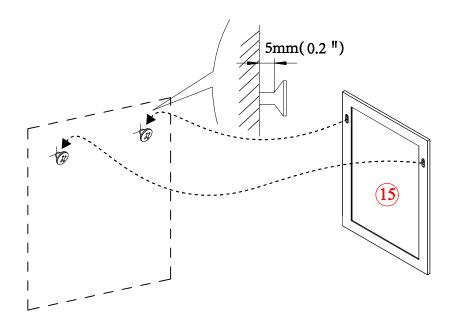
• Insert the expansion into the anchor .Leave about 5mm(0.2") clerrance for the mirror.Then connect the mirror.
