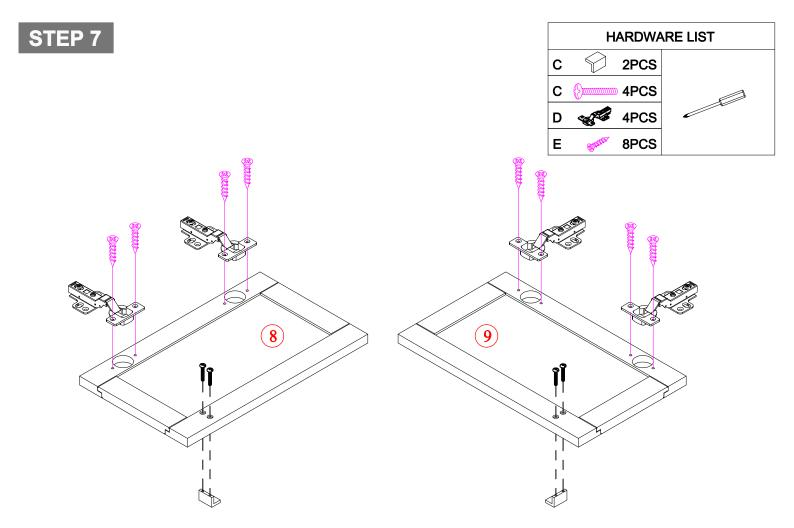
• Use Screws to install the handle and apply Screws to fix the hinge on the shelf #8 and #9.
