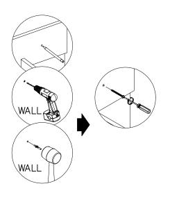
• Refer to the illustration, Draw the spacing between the walls on the cabinet, punch holes in the wall, and fix the cabinet to the wall with screws.
