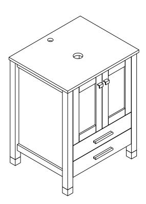
• To help prevent mildew,apply sealant to the space between the wall and the edge of the cabinet.
