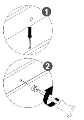
• Insert panel #6 and #7 to their corresponding positions. Then tighten the cam lock.
