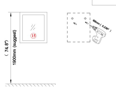
• Measure the distance of hole on the back of mirror and insert the expansion anchor into the wall. **Note:** Appropriate distance from the top of mirror to the ground is 74.8".
