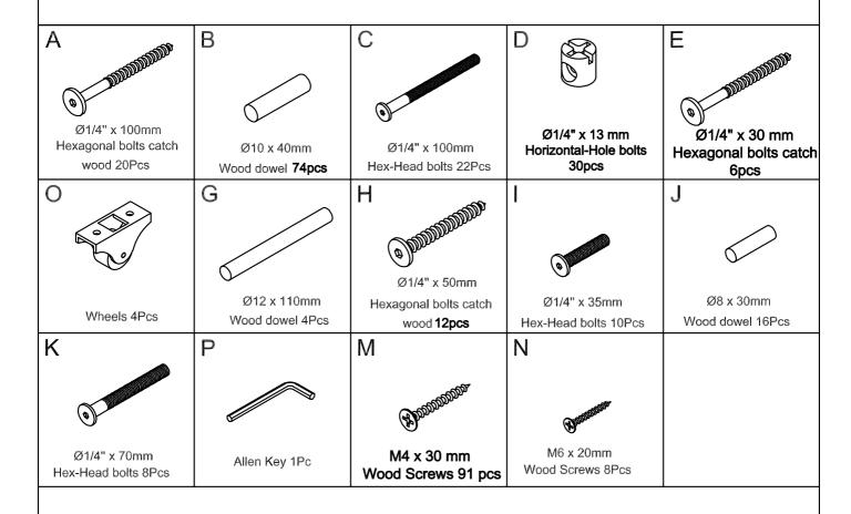
STEP 1 Align and fix Upper legs (1&1.1 & 2) and Upper side panels (3) using Hexagonal bolts catch wood (A) and Wood dowel (B), Tighten with Allen Key (P). STEP 2 Align and fix the guard rails (4 & 5) and the Upper side rail (7 & 8) with the right and left side of the headboard, using Hexagonal bolts catch wood (A) Hex-Head bolts(C) Wood dowel (B) and Hole bolts (D) Tighten with Allen Key (P). (8)08/16
