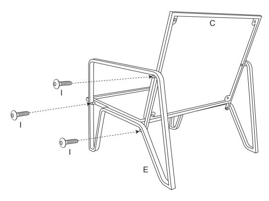
Attached the Right Side Frame (F) to the Back Frame (C) by using Allen Bolt (I) as STEP 3 shown in below diagram. Please 80% tighten the bolts.
