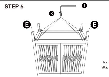
Flip the cabinet upside down and attach the legs using shorter screws.
