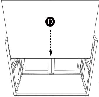
Slide in the back panel between the wood slots on side panels and bottom panel.
