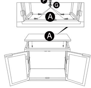
Sit the top panel, open the cabinet doors and attach the top panel to the frame using longer screws.
