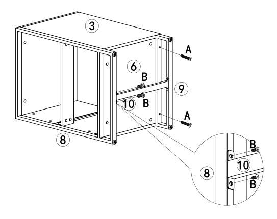
Fully tighten all screws using (L) at this time.
