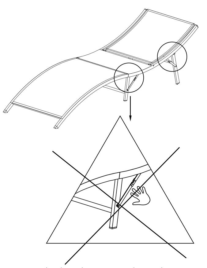
Do not put your hand into the rotating mechanism during merging to prevent hand clamping
