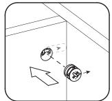
Using a screwdriver, you will turn the cam lock until it stops, usually between 130° or 180°. You will feel the panels pulling closer until they are secured.
