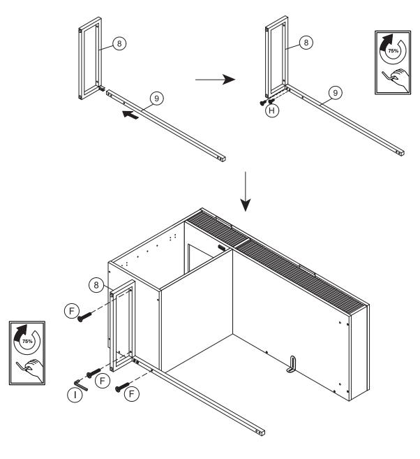
Take the Right Side Metal Frame (10) and attach it to the Top Sub-assembly (1) and the Back Metal Stretcher (9). Use the Ø1/4x12mm Bolts (H), the Ø1/4x32mm Bolts (F) and the Allen Key (I) to firmly secure it in place. Tighten everything to 100%, even those from previous steps.
