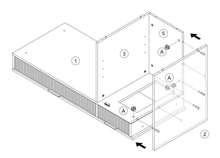
Time to fasten the Left Side Panel (2) into place! Begin by sliding the drawer outward to expose the corresponding holes. Proceed to insert the Ø1/4x28mm Bolts (G) into each hole and tighten them using the Allen Key (I).
