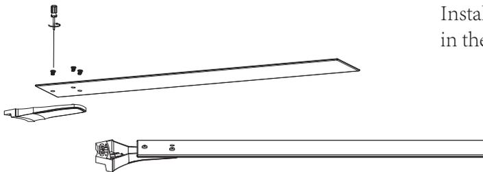
Install the blade holder and blade connection as shown in the picture steps
