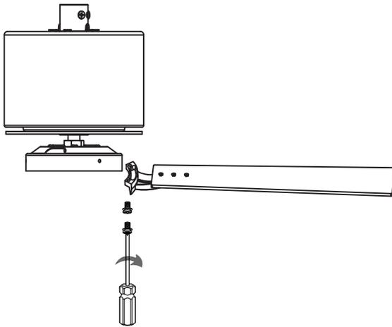
Lock the 8 blade holder components onto the motor
