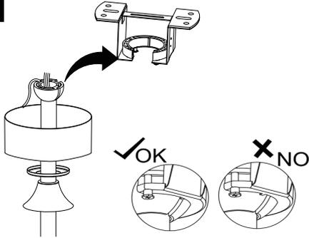
As shown in the figure, the main fan is hung on the hanger plate,
