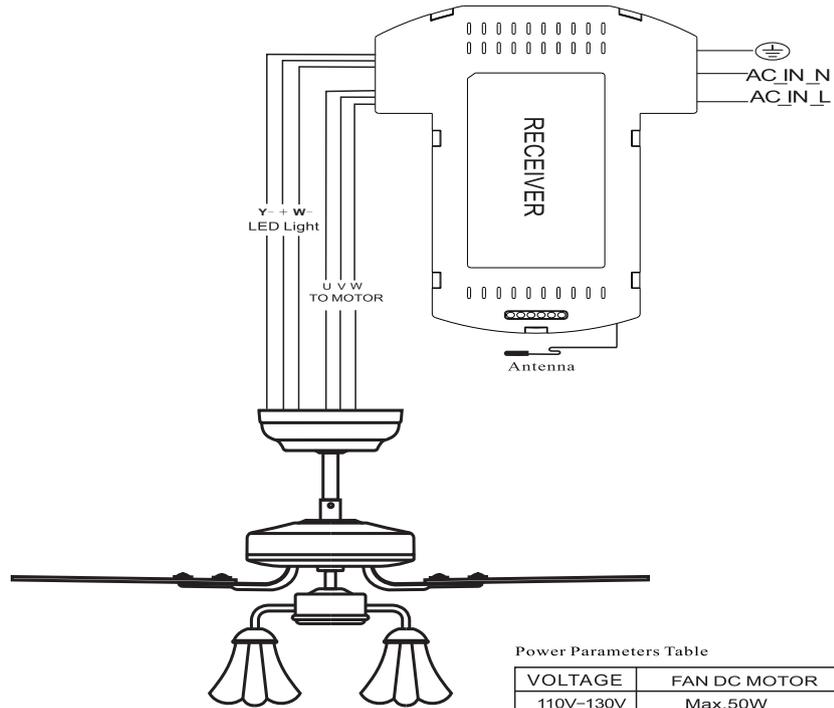
Use wire connecting nuts supplied with the remote controller.
