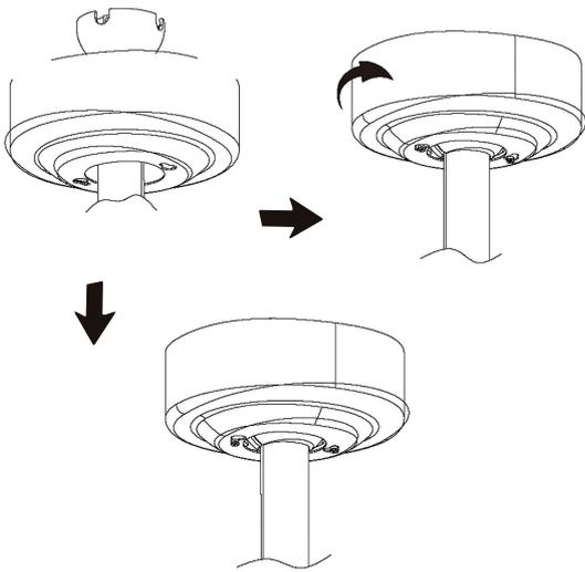
Screw the suspension cup into the two screws below the suspension bracket in the direction of the arrow and tighten them with a cross screwdriver
