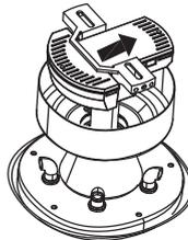
1. Carefully push the canopy to the bottom of the mounting bracket, make two sliding holes aligned to the two prominent screws on the mounting bracket, and then turn clockwise until tight.
