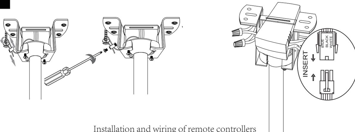
Installation and wiring of remote controllers
