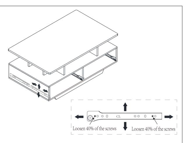
For uneven drawers: Remove uneven drawers and loosen screws on CL/CR rails. Adjust CL/CR rails slightly up, down, forward, or backward. Then tighten the screws to level the drawer.
