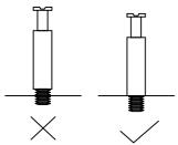
Below shows how the pins are used to assemble the panels together.
