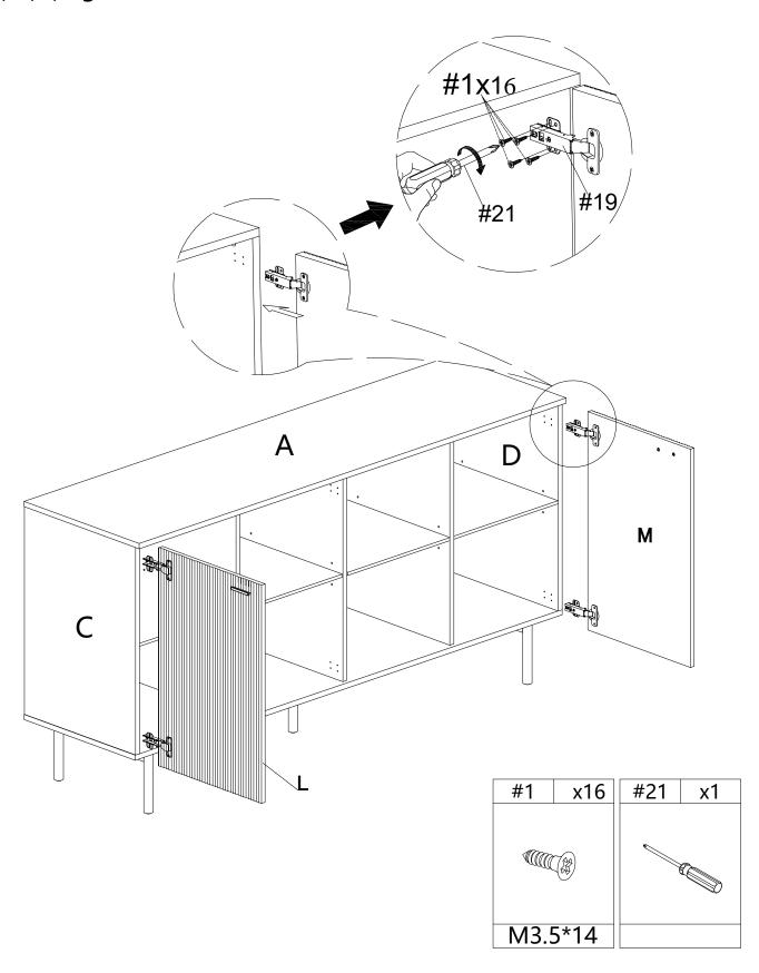
Use screw #1 to attach hinge #18 to door (L)&(M),tighten screw #1 with screwdriver #21.
