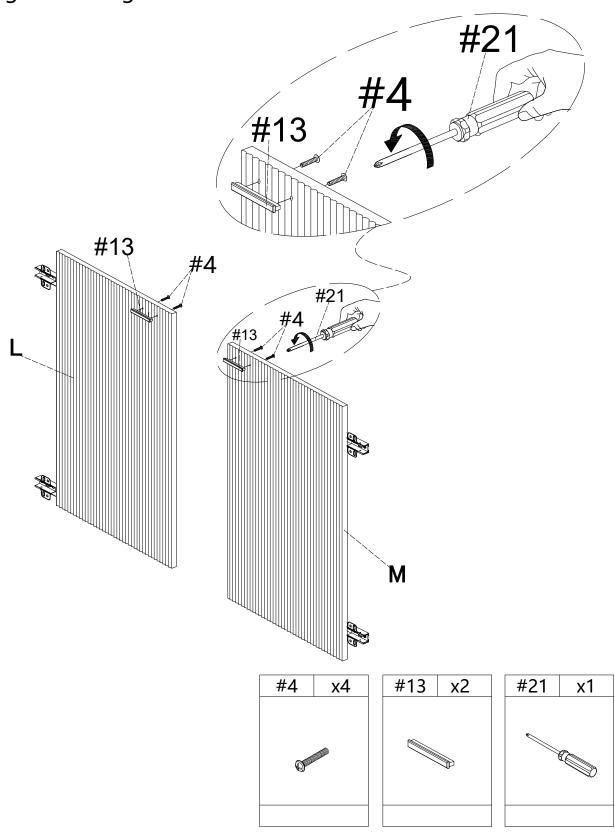
Use screw #1 to attach preassemble door(M)&(L) to panel (D)&(C),tighten screw #1 with screwdriver #21.
