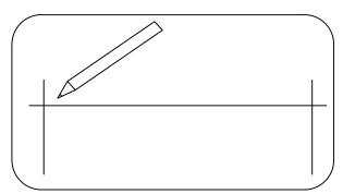
2.Use a pencil to drawflat lines on the wall. The intersection point is the point of punching
