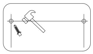
4. Hammer the expansion material into the hole
