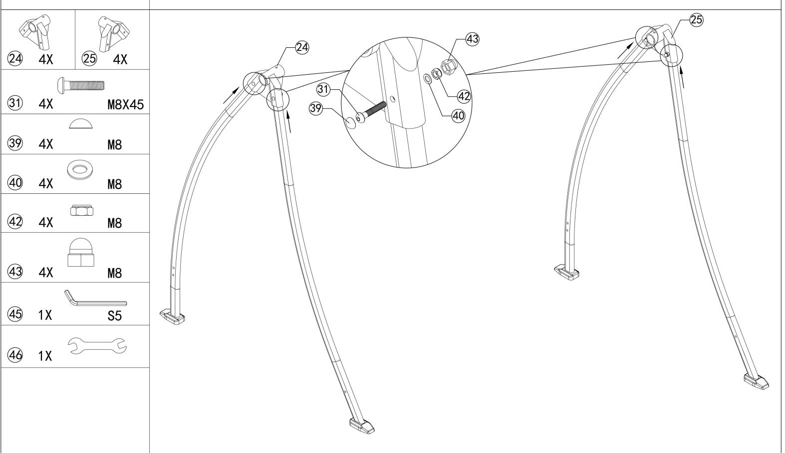
Step 2: Put the front and rear leg tubes (Part 1 is front leg tube, Part 2 is rear leg tube) into the fixator (Part 24 and Part 25) as shown, and secure with bolts and nuts as required (After all the bolts are assembled in place, tighten them together, finally cover the caps).
