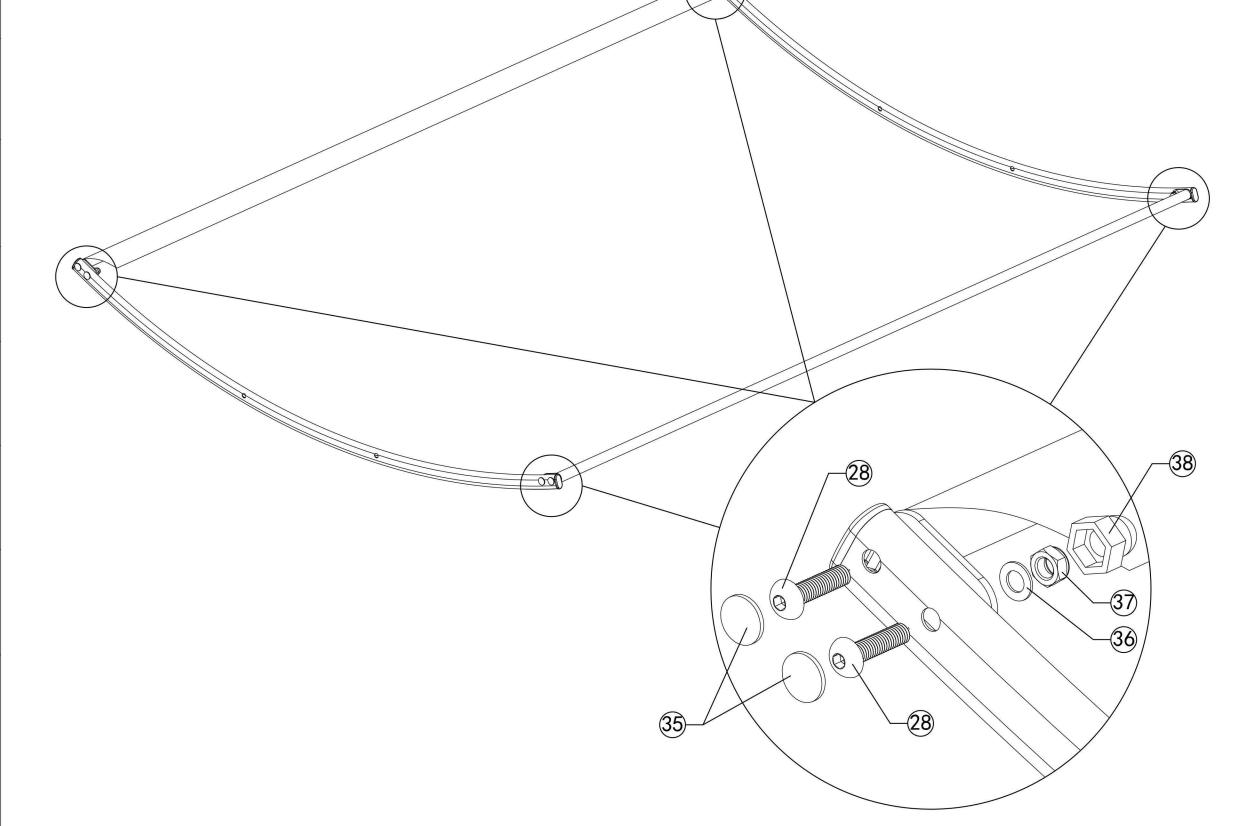
Step 8: Secure the four corners of the canopy with bolts and nuts as required (After all the bolts are assembled in place, tighten them together, finally cover the caps).
