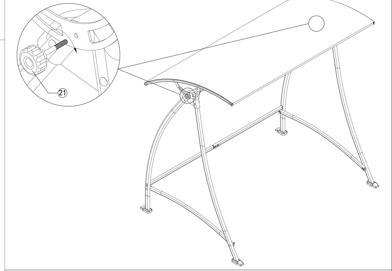
Step 10: Fix the canopy on the assembled leg frame with the adjusting knob (Part 21) as shown. Attention: According to your own requirements to adjust canopy roof, then tighten the knob.
