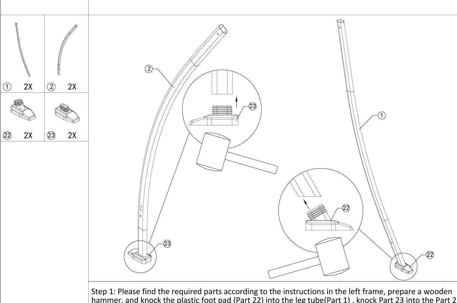
Step 1: Please find the required parts according to the instructions in the left frame, prepare a wooden hammer, and knock the plastic foot pad (Part 22) into the leg tube(Part 1), knock Part 23 into the Part 2 as shown.
