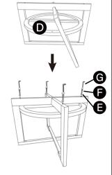
Attach the bottom shelf D to wood base by bolts and flat washers as shown above.
