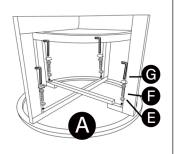
Attach wood base B and C to the bottom of table top A by bolts and flat washers as shown above.
