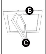
Attach wood base B to wood base C as shown above.
