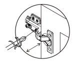
This is used to adjust the door panel in the up and down direction.
