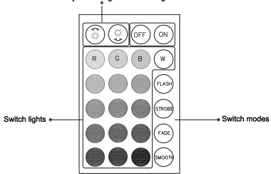
Please note that for transportation safety, the remote control does not contain batteries; the attery model is: CR2025
