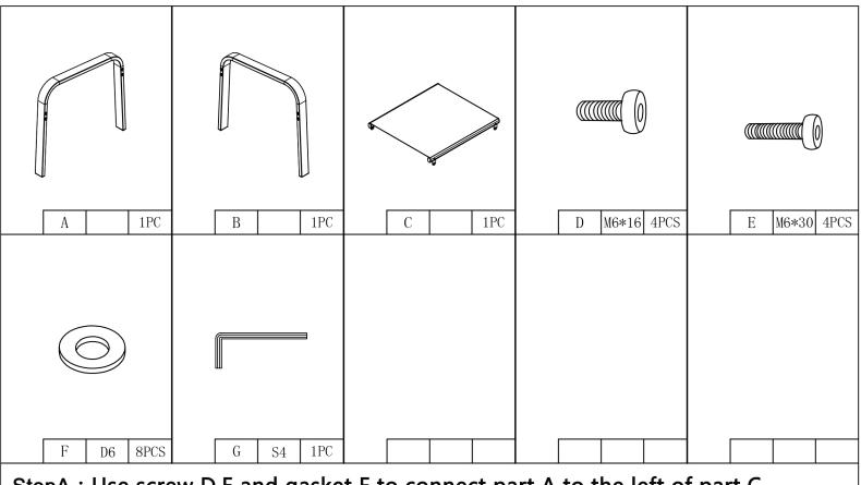
StepA: Use screw D,E and gasket F to connect part A to the left of part C.
