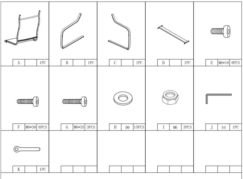
StepA: Install screw G and gasket H & I as shown in part A. (Please don't tighten the screws until the last step.)
