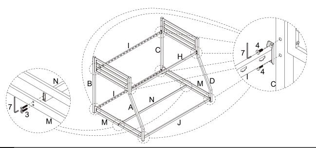
Insert Slat (K & L) into Rail (H, I, J) as shown. Then lock Slat Connector (P) to fix Slat (K & L).
