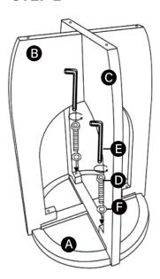
Interlock the female leg C in the wood slot and attach to bottom of table top A.
