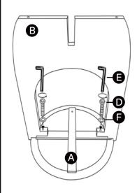
Flip table top A upside down. Attach male leg B to the bottom of table top A.
