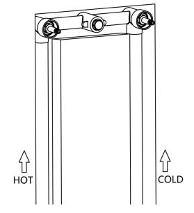
3. Fix the main body of the faucet with self-tapping screws (the main body must be flush with the wall).
