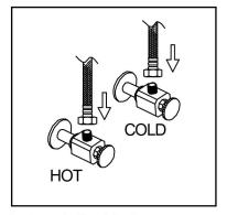
4. Attach flexible hose to water supply.
