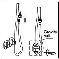
3. Connect the pull tube to the quick connect water outlet pipe, and then install the gravity ball at a position about 100mm/4" from the bottom. Repeat several times to pull the sprinkler head back. If there is no jam, it can be used.
