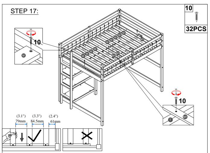
Note: Do not lock the screws of the bed slats to the outermost edge of the bed slats, you need to leave a certain space at the edges, otherwise it will cause the board to break. Do not lock the bed slats on the edge of the wood, please hold firmly before screwing,
