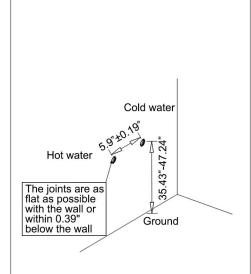
1, An first to ensure that the two out in the same level and ensure that the distance between the two outlets in the deviation in the allowable range according to the left hot right cold method connected to the hot and cold water source Flush the debris in the water
