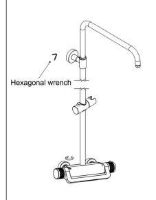
7, Rotate and fix the shower tube assembly on the main body, and then fix the tube set on the fixed base with a hex wrench.
