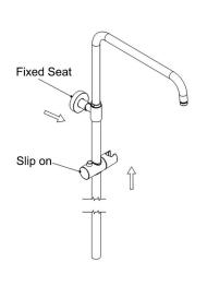
4, Slip the slide set into the shower pipe set, and put the fixed seat on the shower pipe set
