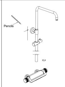
5, Rotate the shower tube and fix it on the body, then mark the fixing position of the fixing seat.
