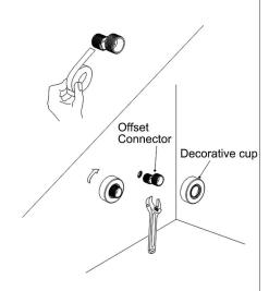
2, Wrap the appropriate amount of raw material tape around the threads of the curved foot and use an adjustable wrench to install the two curved feet wrapped with raw material tape on the water pipe and then screw in the decorative cover
