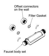
3, Use the installation positioning tool curved foot center distance and level to assemble the body on the filter gasket after fixed on the curved foot Test the water with 0.5Mpa water pressure, confirm no leakage and then install the shower pipe set
