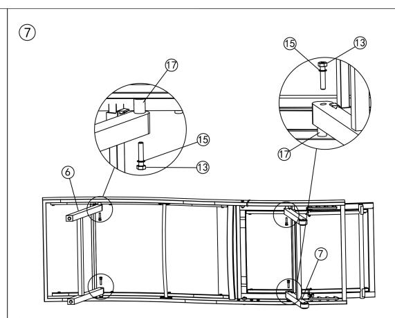
**Step 7**: Install Front Leg (Part 6) and Rear Leg (Part 7) to Bedframe using Plastic Cylinder (17), Bolt (13), and Washer (15).
