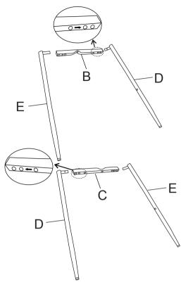
Please fix the Legs to Criss-Cross Supports as shown in below diagram by using STEP 2 Allen Bolt (G) and Allen Wrench (K), Please tighten the bolts to 90%.
