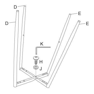
STEP 4 Attach the Legs (D&E) to the Seat (A) as shown in below diagram by using Allen Washer (J), Allen Bolt (I) and Allen Wrench (K), Please tighten the bolts to 90%.
