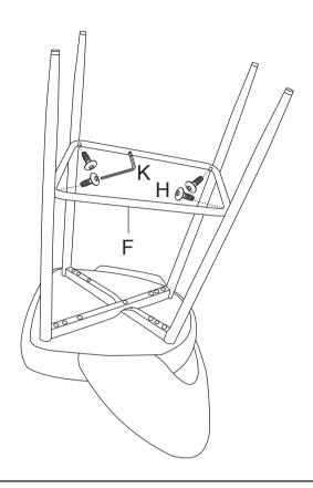
STEP 6 In this step please make sure the chair legs are flat and all bolts are installed, then please tighten all bolts to 100%.
