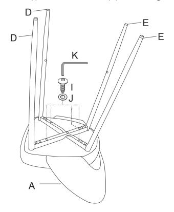
STEP 5 Attach the Footrest (F) to the Legs (D&E) as shown in below diagram by using Allen Bolt (H) and Allen Wrench (K), Please tighten the bolts to 90%.
