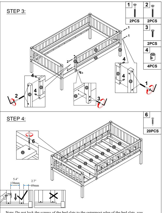
Note: Do not lock the screws of the bed slats to the outermost edge of the bed slats, you need to leave a certain space at the edges, otherwise it will cause the board to break. Do not lock the bed slats on the edge of the wood, please hold firmly before screwing, hold it in place with one hand, then lock the screw.
