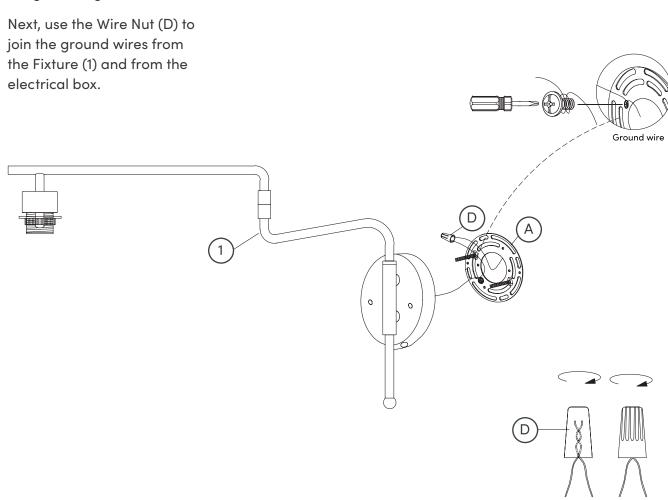
Feed the designated wires into their respective wire connectors, as shown below. Attach Fixture (1) to the Mounting Unit (A). Align the holes on the Fixture with the exposed screws. Tighten them securely using the Finial Nuts (B). Turn the Finial Nuts (B) in a counter-clockwise direction. Unscrew the collar fitting from the Fixture (1) by turning it clockwise until it comes off.
