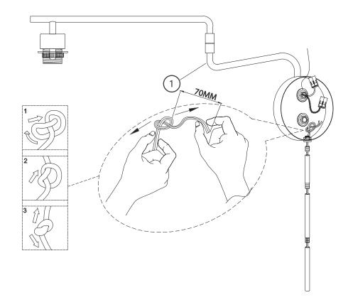
To proceed, open the flaps once again. Insert the clear neutral wire alongside the white wire. Place the hot wire (marked with an L) next to the black wire.
