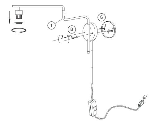
Install the Shade (2) by setting it in place with the shade collar fitting that you removed in step 14.
