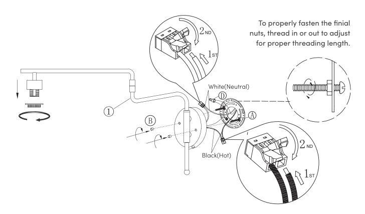
Install the Shade (2) by setting it in place with the shade collar fitting.
