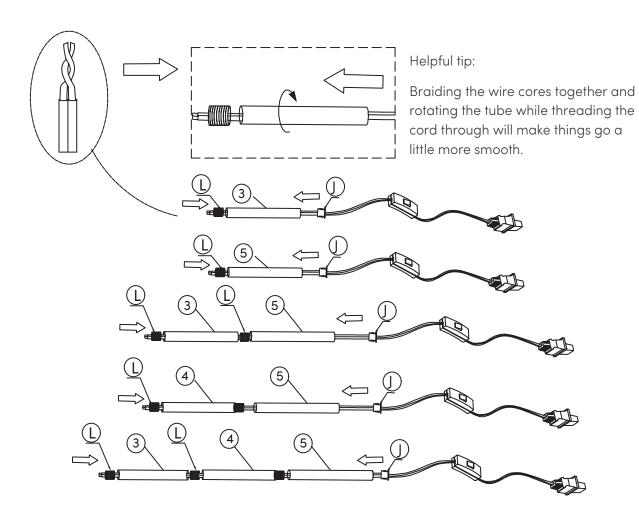
Take the wires and guide them back through the hole at the bottom of the Fixture (1) – it's like threading a needle.
