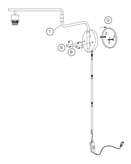
Carefully raise the flap on the wire connector to release the clear wire. Repeat this step on the second connect so that both clear wires have been removed and the black and white wires remain attached to the Fixture (1).
