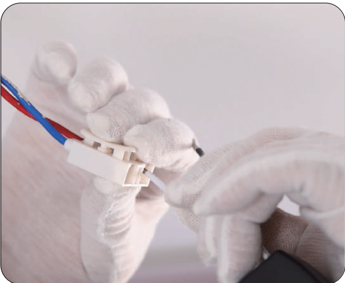
21. Connect the Receiver-1
