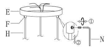
5 » If needed, shorten the extra length of the fixture wires from cords (H) so that they all are at least 6 inches (152.4 mm) long above canopy (E) within the outlet box.
