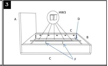
**STEP 3:** Insert the center support rail(D) in the metal brackets on the Headboard(A) and Footboard(B). Adjust the feet on the metal legs(F) so that they are resting evenly on the floor. Put the plastic cap(HW3) in the center support rail(D) evenly.
