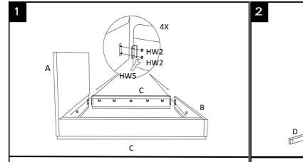
**STEP 1:** Attach the Siderails(C) to the Headboard(A) and Footboard(B) by the nuts(HW2) and wrench(HW5).
