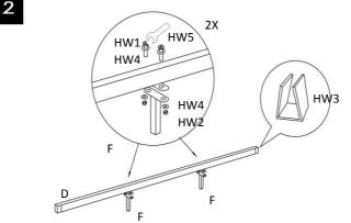
**STEP 2:** Screw the 2 metal legs(F) onto the long iron center support rail(D). Insert the plastic cap(HW3) in the iron center support rail(D).
