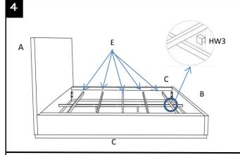
**STEP 4:** Insert the remaining 5 iron slats(E) horizontally between the left and right Sideboards(C). Make sure the plastic caps(HW3) between the center support rail(D) and each of iron slats(E).
