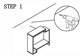
1. Find spot on wall 1" below top of item. 2. Using a drill bit slightly thinner than anchor , drill hole into drywall.
