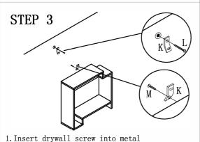
bracket and into drywall anchor.
