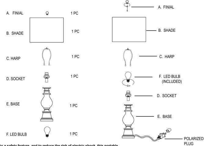
As a safety feature, and to reduce the risk of electric shock, this portable lamp includes a polarized plug (one blade is wider than the other). The plug will fit into a polarized outlet in a single direction only. If the plug does not fit fully in the outlet, reverse the plug and try again.
