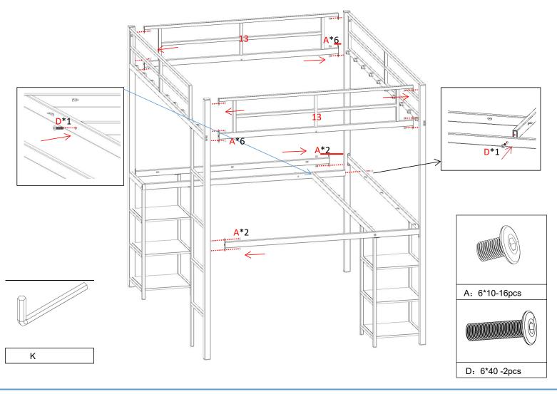
Step 8: Using hardware D,K connect #15.
