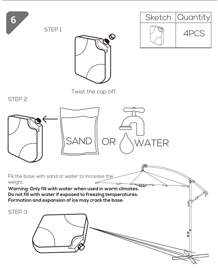
Place the water or sand filled base snug into a corner of the umbrella stand as shown in the diagram. Note: It is recommended to use 4 plastic bases to properly weigh the umbrella base to the ground.
