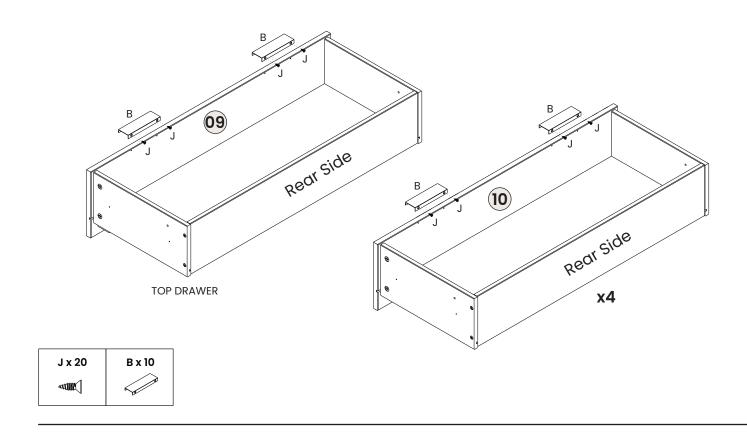
Before to fix the Drawers, you must extract the full extension of the Slides, by pulling off. Then, pay attention to the correctly holes according to the next steps.
