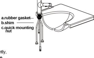
Note: please pass the hot and cold water pipe with hexagon nuts through the dental tube nuts one by one, and then put the hose with quick connect fitting through the dental tube nut.
