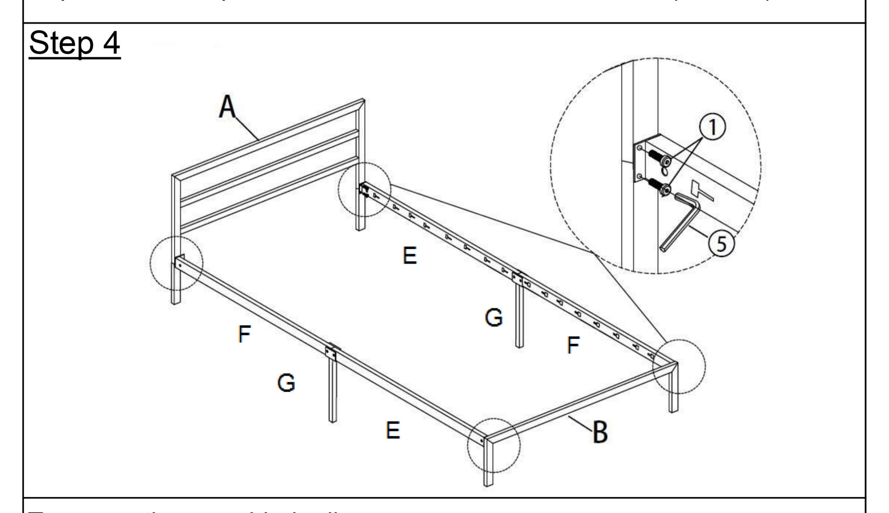
Turn over the asembled rails. Attach Side Rail frame(E&F&G) to Headboard(A) and Footboard(B) using Bolt(1) with Allen Wrench(5).
