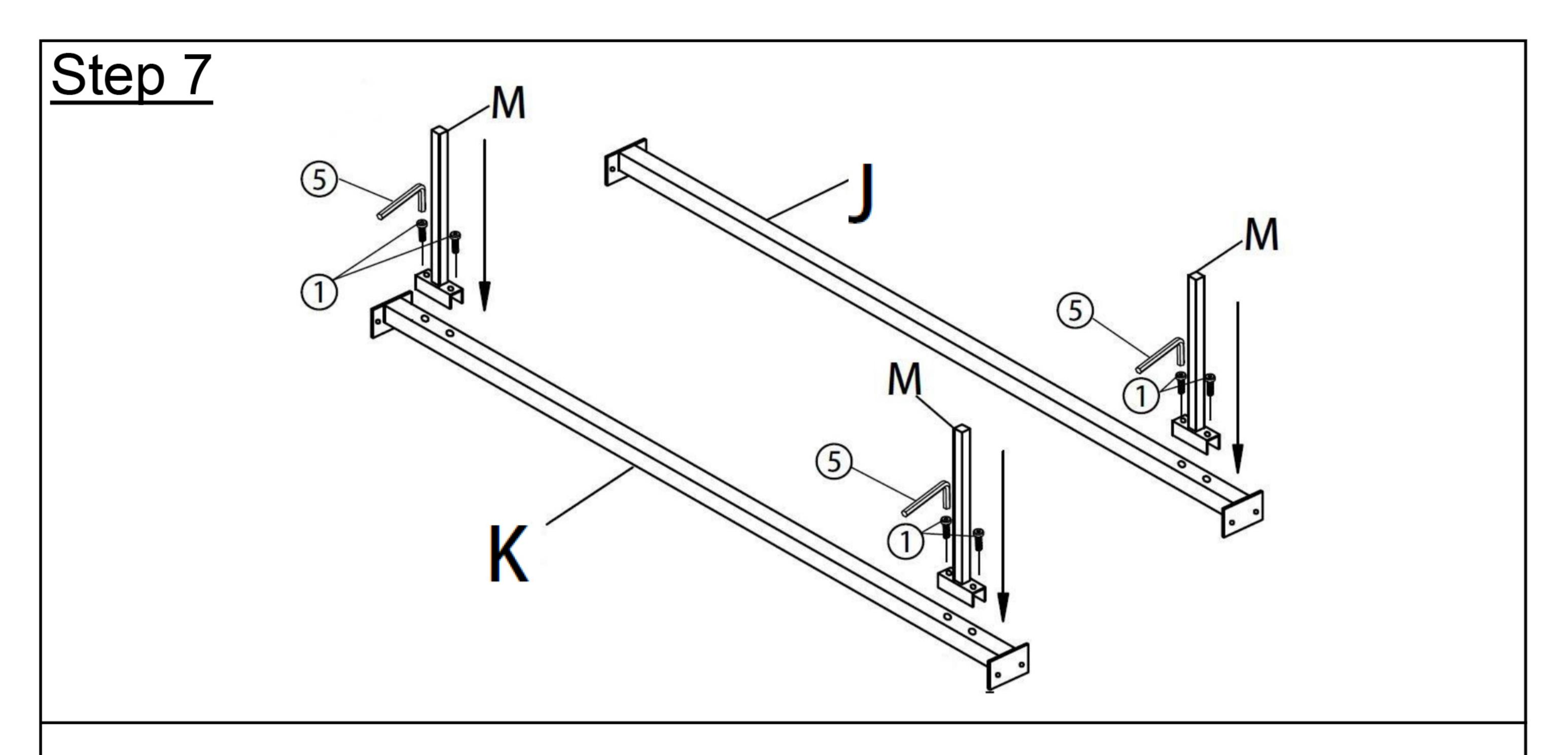
Align the mounting positions of Support Leg(M) to Vertical Front Center Rail(J).
