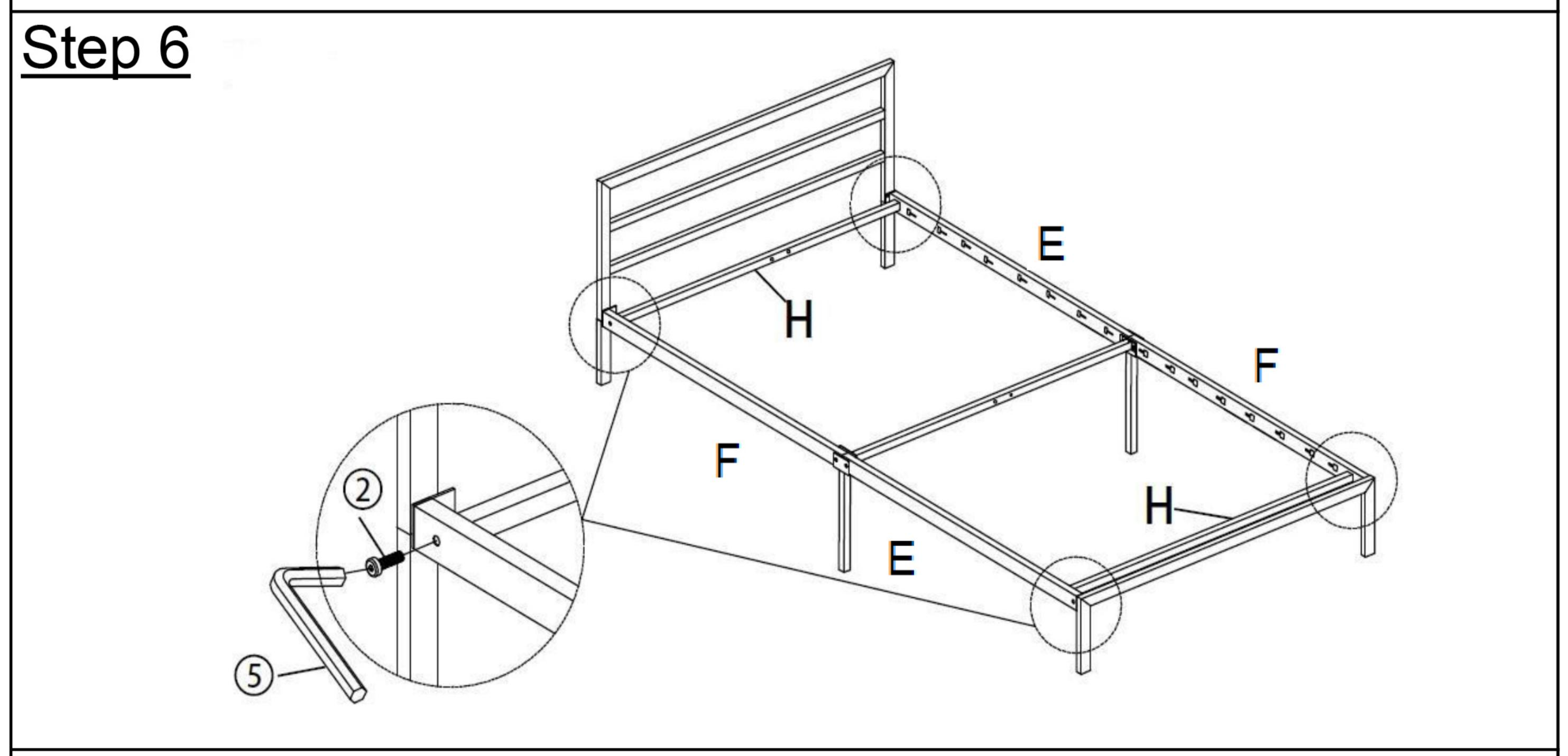
Attach Support Rail(H) to Side Rail(E&F) using Bolt(2) with Allen Wrench(5).
