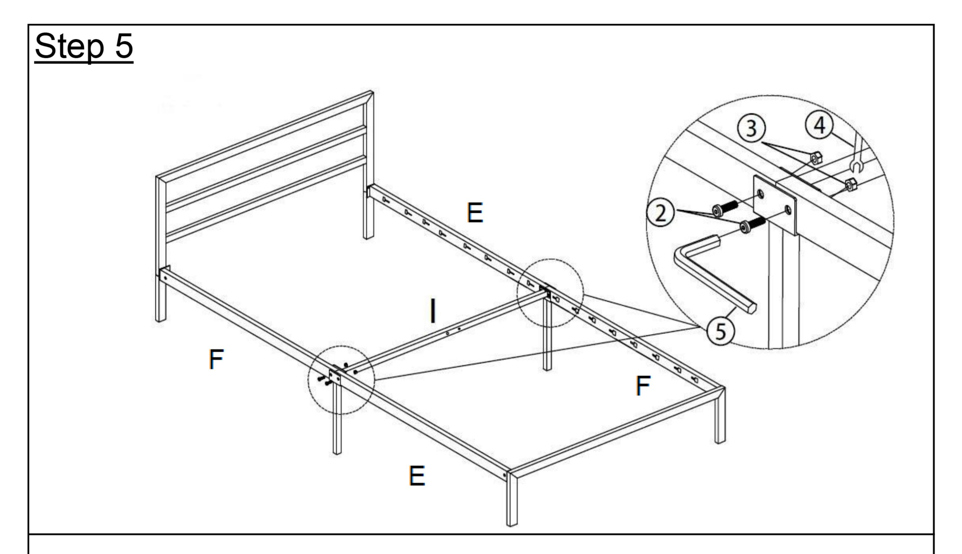
Attach Cross Center Support Rail(I) to the Rail(E&F) using Blot(2) and Nut(3) with Allen Wrench(5)and Wrench(4).
