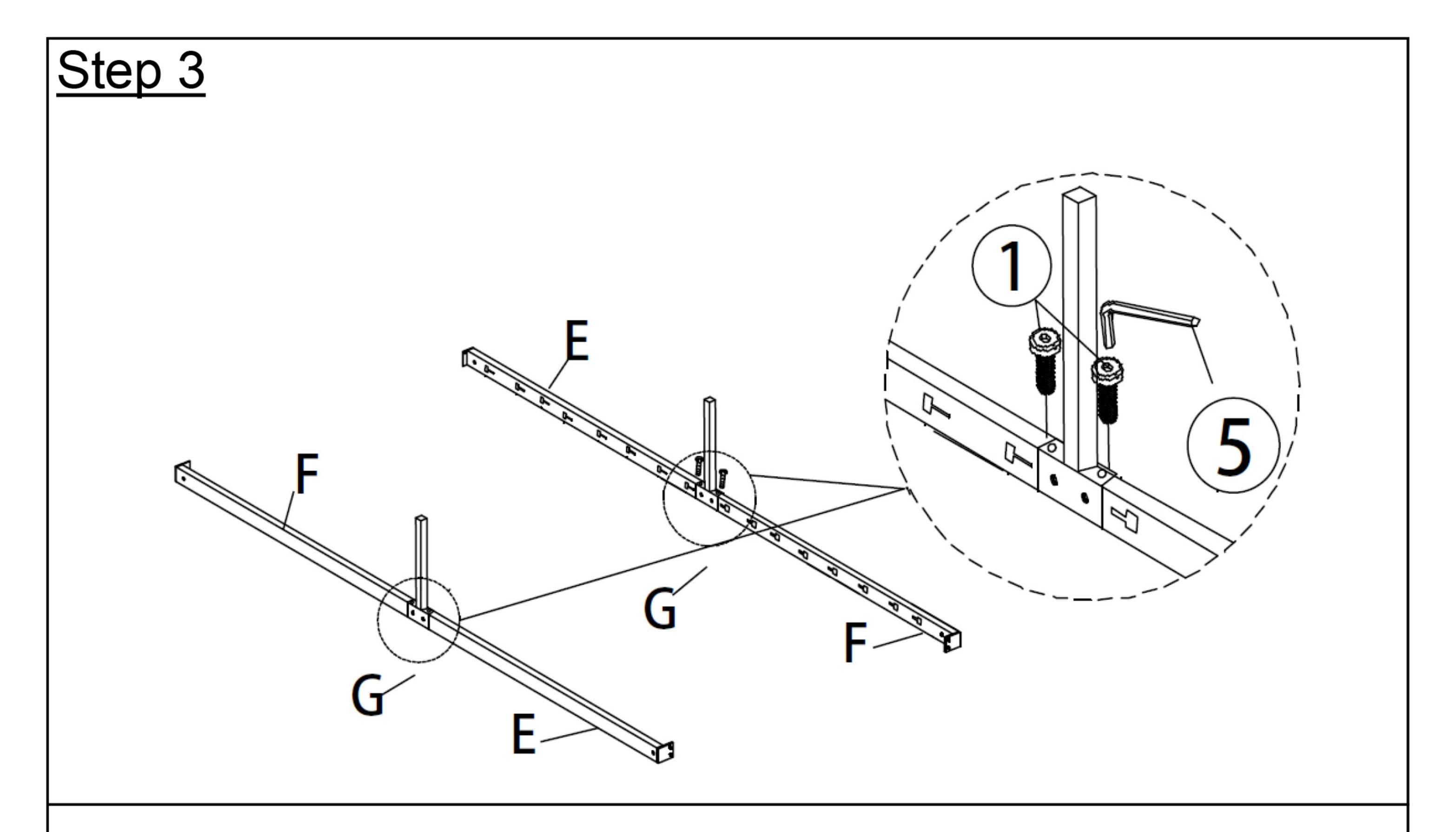
Align the mounting positions of Rail Support Leg(G) to Side Rail(E&F). Attach Rail Support Leg(G) to Side Rail(E&F) using Bolt(1) with Allen Wrench(5).
