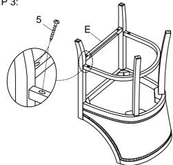
1.Loosely attach the Front stretcher (E) to the Left (B) and Right Left (C), using Screw (5) with a Philips head screwdriver to tighten, as shown.
