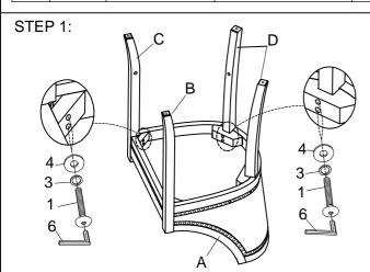
1. Loosely attach the Left Leg(B) and Right Leg(C) to the Fabric Seat(A), using Bolts(1+3+4) to tighten, as show. 2. Loosely attach the two Back Legs(D) to the Fabric Seat(A), using Bolts(1+3+4) to tighten, as show.
