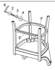
1.Loosely attach the Back Stretcher (F) to the Back leg (D), using Bolts (2+3+4) to tighten, as shown.
