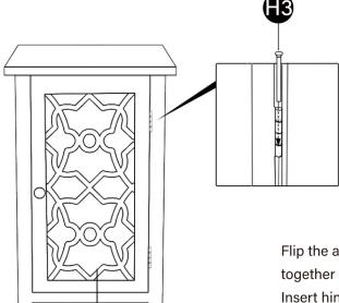
Flip the assembly. Align the hinge leafs together on door panel H and right panel B. Insert hinge pin H3 through the hollow knuckle.
