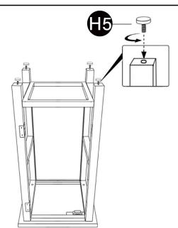
Screw in levelling feet and adjust as needed.
