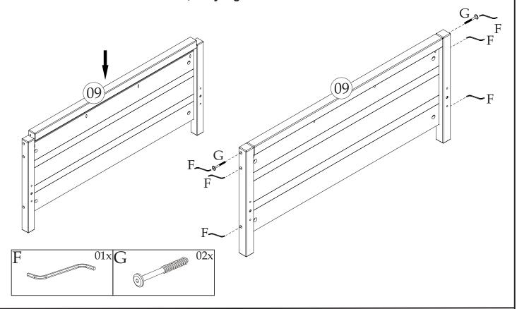
Step 13 - Attach Foot Board Lower Cross Rail (Part 12) to Bed Posts (Parts 03 & 04) using the 4 x Screws "BW". Screw in "AR" screw into Footboard posts (Parts 03 & 04) – as shown in drawing.
