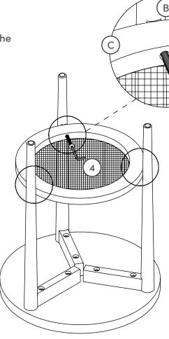
Do NOT overtighten hardware. Tighten only 75% for now.
