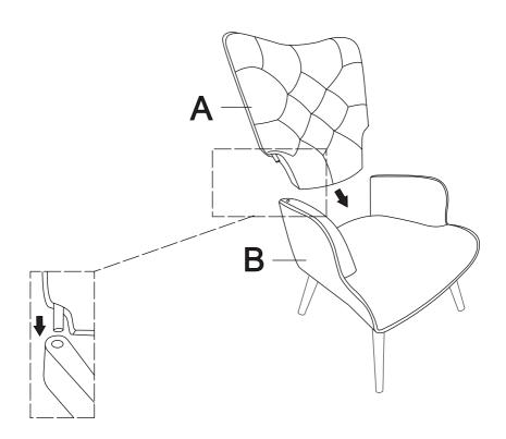
There are 2 plugs on the bottom of the Seat Back(A), and 2 holes on the armrests of the Seat Bottom(B).
