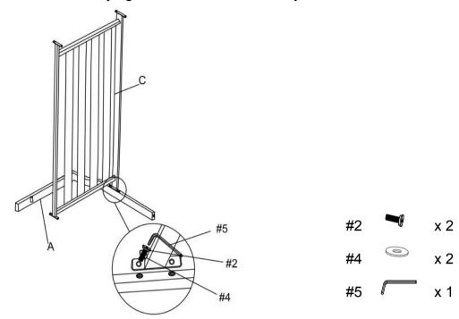
Step 2. Attach left arm (part B) to seat panel (part C) using bolts (part #2), flat washers (part #4) and allen wrench (part #5).
