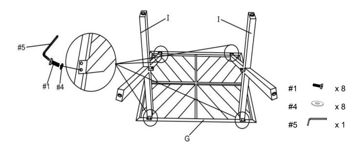
Step 6. Attach table connector (part H) to table legs (part I) using short bolts (part #1), flat washers (part #4) and allen wrench (part #5).
