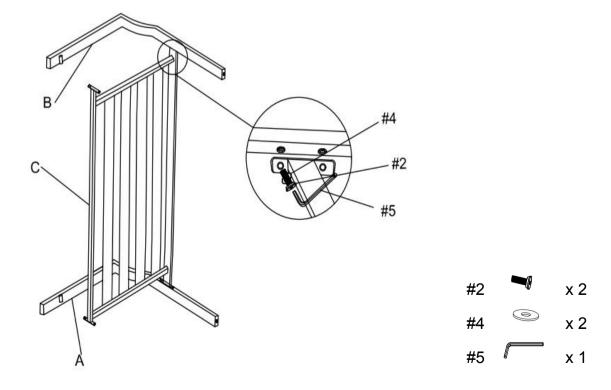
Step 3. Attach back panel (part D) to assembled unit (parts A, B & C) using bolts (part #2), long bolts (part #3), flat washers (part #4) and allen wrench (part #5).
